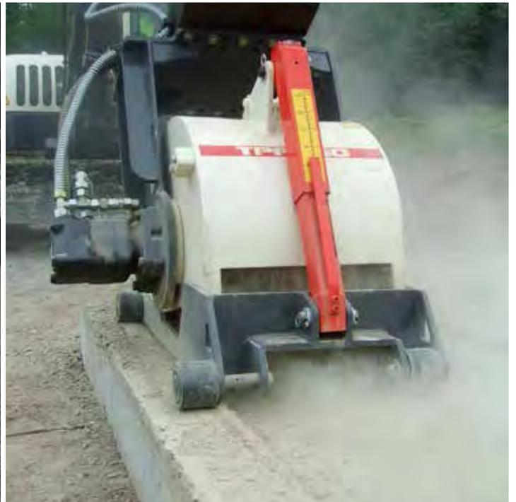
**CUTTING DEPTH CAN BE CONTINUOUSLY ADJUSTED**
