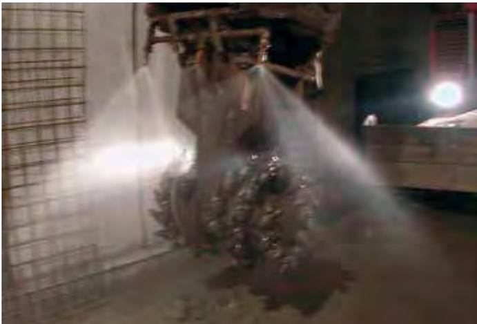
**Water spray unit to damp down dust**
